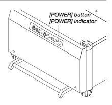
**NOTE:** Immediately after turning on the projector, screen flicker may occur. This is not a fault. Wait 3 to 5 minutes until the lamp lighting is stabilized.
